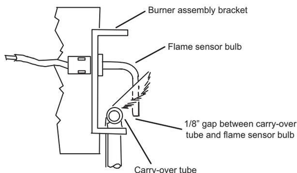
**Figure 27: Proper Flame Adjustment**
