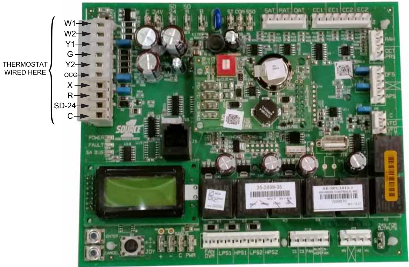
Figure 30: Unit Control Board
