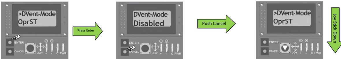
**Step 5** - By pushing the joystick down, the cursor toggles to OprST (Operating Space Temp).
