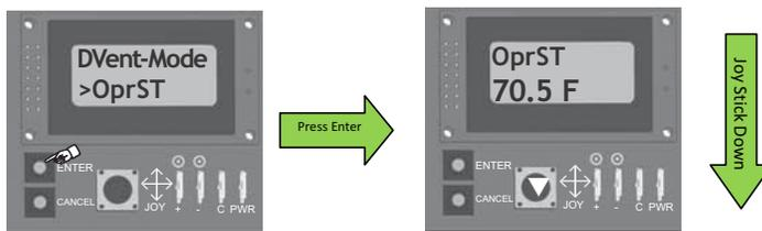
**Step 6** - By pushing "ENTER" the actual OprST (Operating Space Temp) appears. Pushing the joystick down scrolls through SAT, RAT, OAT and other available sensor readings.
