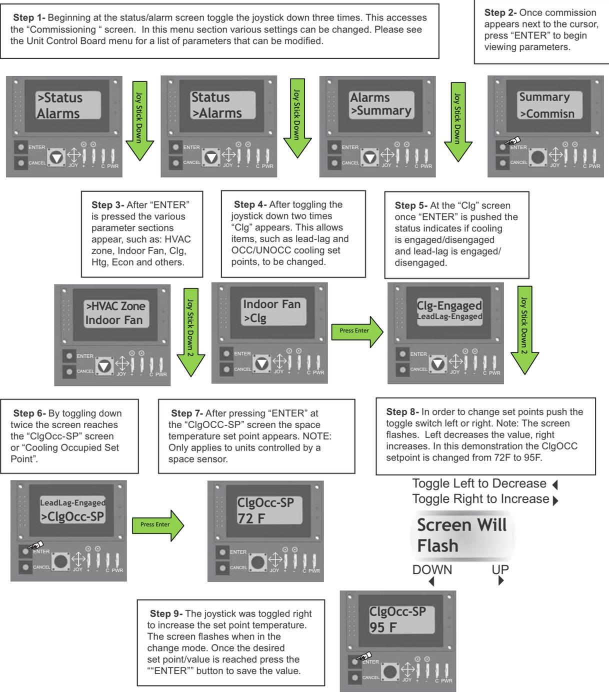
These few pages provide a simple demonstration how to navigate the menu's of the Simplicity SE control containing Version 3 firmware. Please utilize this document along with the additional information in the Users Guide and detailed navigation menu to adjust the control to customer preferences or job specifications.
